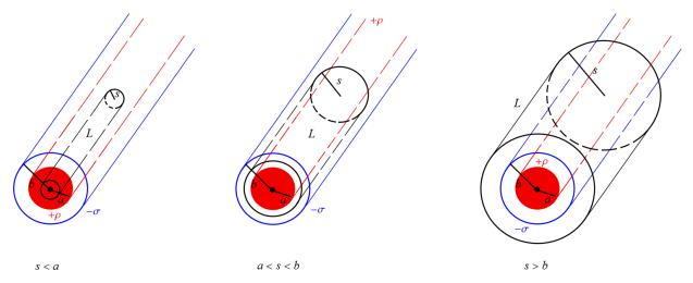
The enclosed charge is the product of the charge density with the volume.
